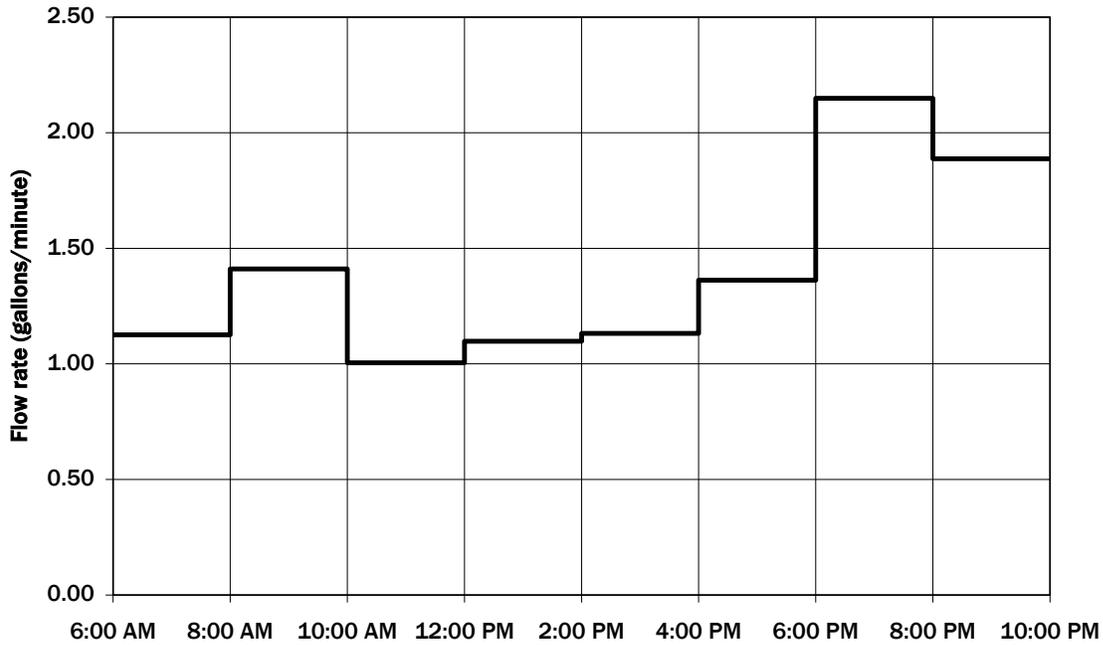
**Figure 9: Average freshwater consumption rates over a day**
