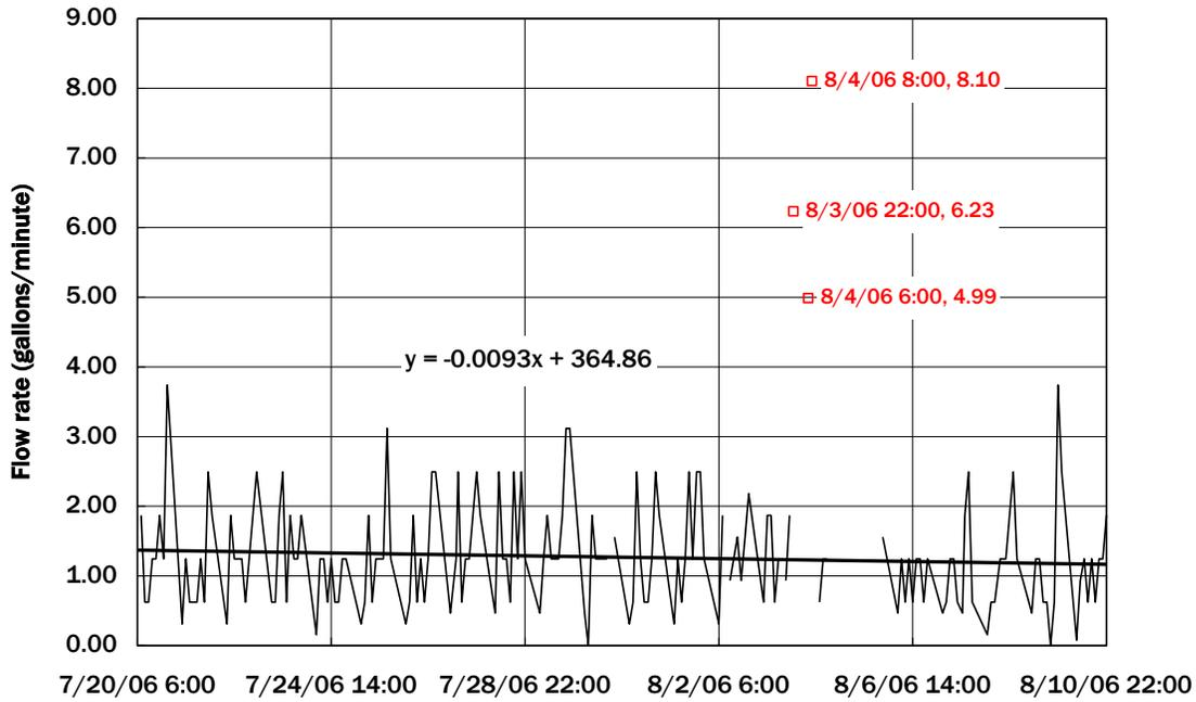
**Figure 7: Freshwater consumption rate over entire collection period**
