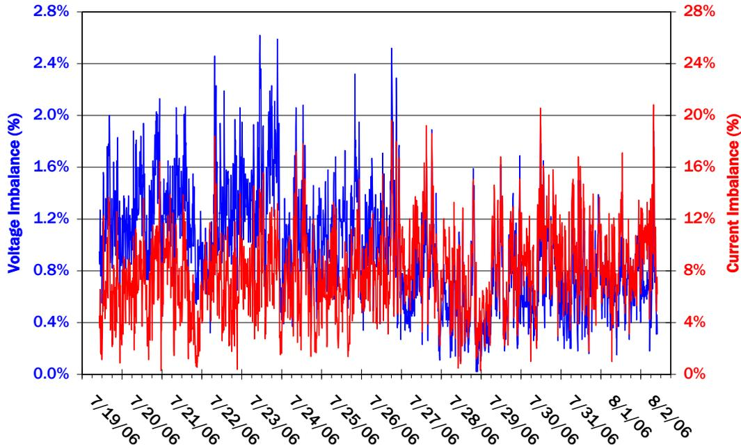
**Figure 15<sup>21</sup>: Comparison of voltage and current imbalance of the generator room 480 V main distribution panel July 19-August 2**
