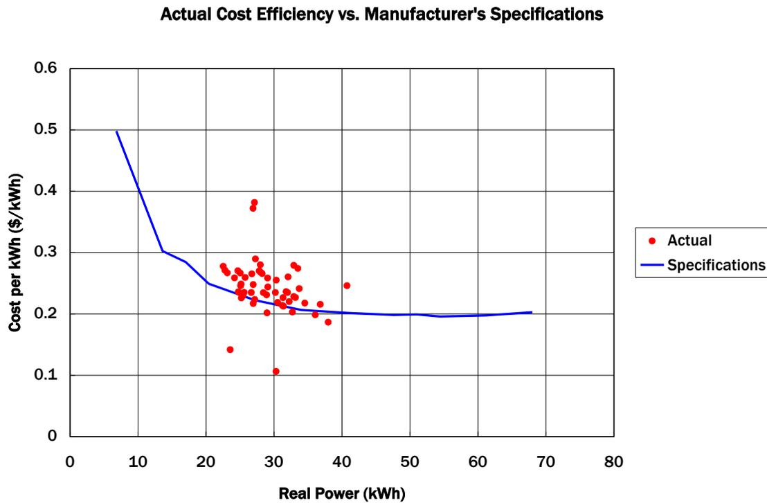
**Figure 17: Comparison between actual cost efficiency from July 20-26 and fuel efficiency based on manufacturer-provided specifications**
