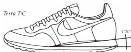
The Air-Sole® (top) in the Columbia, Aurora and Tailwind has different air pressure in the various sizes to give more appropriate cushioning. The Terra T/C (below) has a Phylon™ midsole also scaled for cushion as well as the same degree of heel lift in all sizes.
